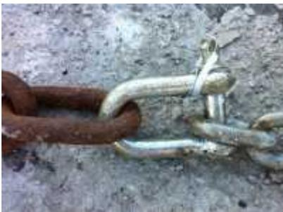
Shackle joining riser chain to ground chain. Note araldite, Monel wire and cable tie used.
