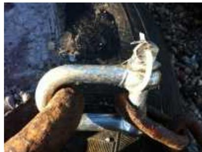
Shackle joining concrete weight to ground chain. Note araldite, Monel wire and cable tie used.
