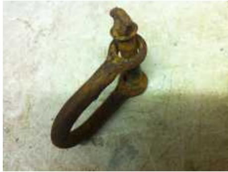
Corroded shackle showing how the pin can become loose. Araldite in this area can help prevent this
