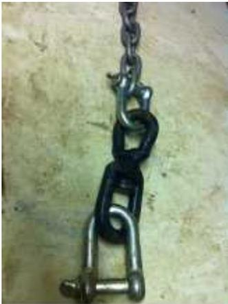
Swivel joining riser chain. Note the size of swivel and shackles relative to chain size
